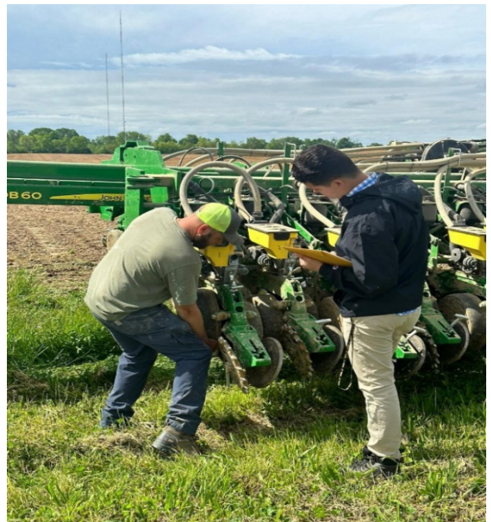
Figure 5. Field execution of TPM checklist on seeding machinery.
